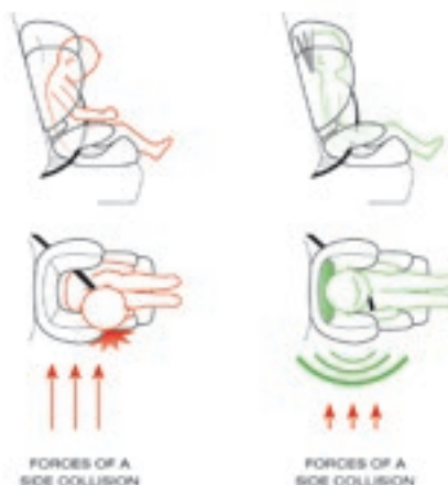
AVERAGE HEADREST VS PATENTED RECLINING HEADREST
